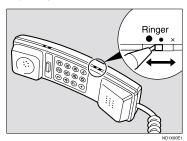
Adjust the handset ringer volume using the volume switch.
